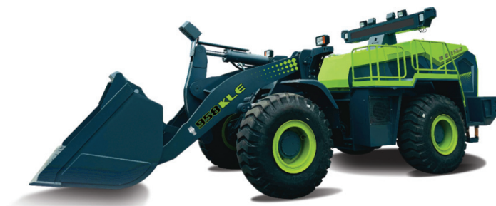
BRT958KLe, our first cabinless remote-operated loader
