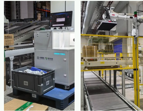
Sinopharm Logistics AI Visual Recognition – Robotic Arm with Intelligent Control Technology for Picking
