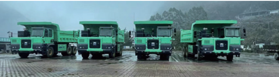
Electric unmanned mining trucks at Hezhou Industry Park
