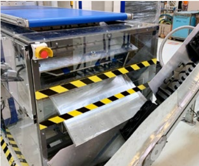
New machine installed to shred waste plastic foil for reuse in the production process
