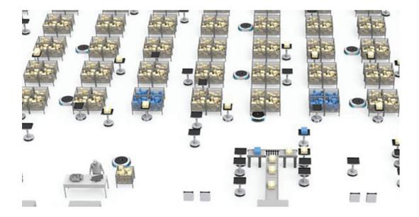
The Geek+ FleetSort Solution addresses end customers' challenges by providing a fully automated process for sorting and handling, from sorting to the final container exchange and outbound dispatch. By combining intelligent sorting robots with goods-to-person picking robots, the solution eliminates the need for manual operations in the box collection and
