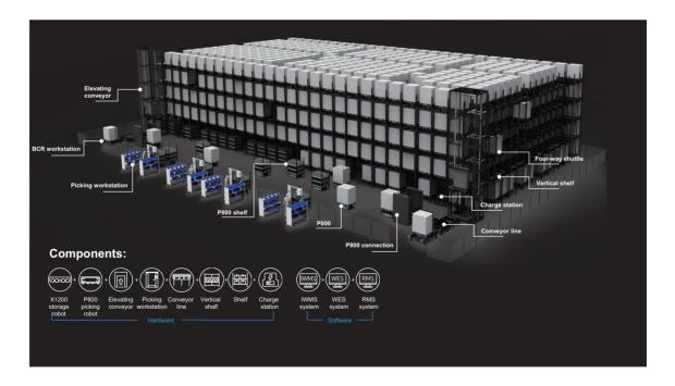
The Geek+ Pallet-to-Person Picking Solution addresses end customers' challenges by offering storage capacity 5 to 8 times higher than ground storage and more efficient than traditional AS/RS systems. It also improves picking efficiency compared to manual warehouses. The integrated RMS system coordinates multiple devices and supports the concurrent operation of thousands of robots, enhancing overall system performance and scalability.
