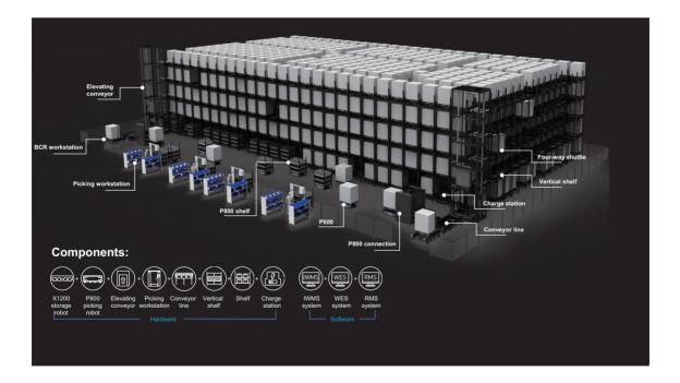
The Geek+ Pallet-to-Person Picking Solution addresses end customers' challenges by offering storage capacity 5 to 8 times higher than ground storage and more efficient than traditional AS/RS systems. It also improves picking efficiency compared to manual warehouses. The integrated RMS system coordinates multiple devices and supports the concurrent operation of thousands of robots, enhancing overall system performance and scalability.
