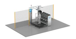
Safety Door . . . . During cleaning or anomaly handling operations, an interlocking guard with guard locking controlled by a safety PLC is utilized to ensure the safe entry and exit of personnel in the robotic area.
