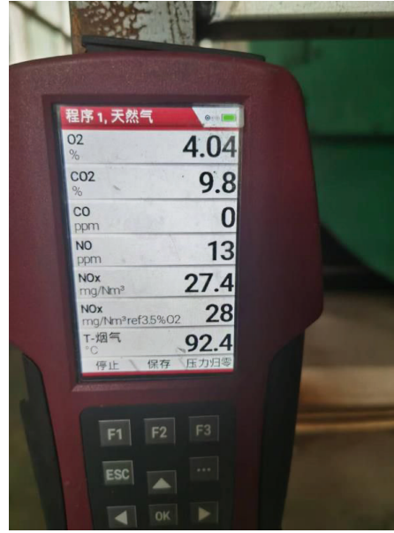
4T Boiler retrofitted with low Nitrogen Oxides burner
