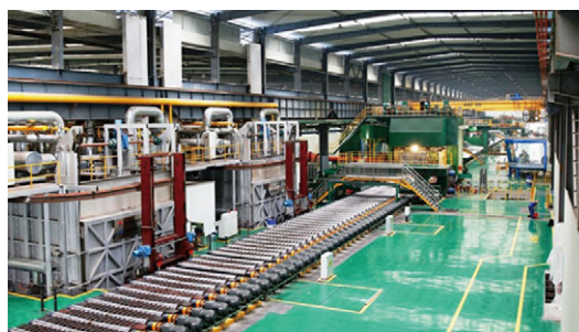
Key technology and equipment development for the 3,300/2,800 twinstand aluminum plate and strip hot rolling mill (1+1 production line)
