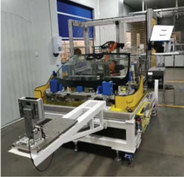
The flexible testing platform provides highly adaptable and precise testing services for the automotive glass industry, which can measure the surface quality and PVB angle through customized testing solutions and in-house developed software algorithms. Our flexible testing platform is compatible with multiple types of glasses and HUDs.
