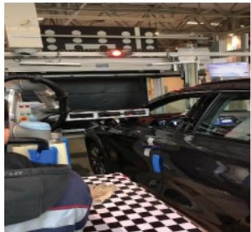
The HUD collaborative robot testing platform is China's first integrated solution specifically designed for automotive HUD and ADAS testing and calibration. This platform innovatively combines collaborative robot technology, enhancing testing efficiency and accuracy, and provides the automotive industry with an advanced quality control tool.
