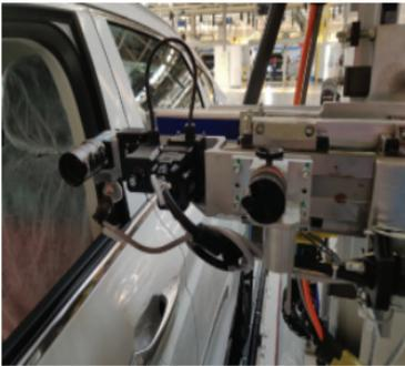
The vehicle end-of-line (EOL) testing equipment utilizes advanced optical testing technology, featuring highly flexible body posture compensation that adapts to various vehicle models' distortions and performs real-time online correction, ensuring testing accuracy and efficiency.
