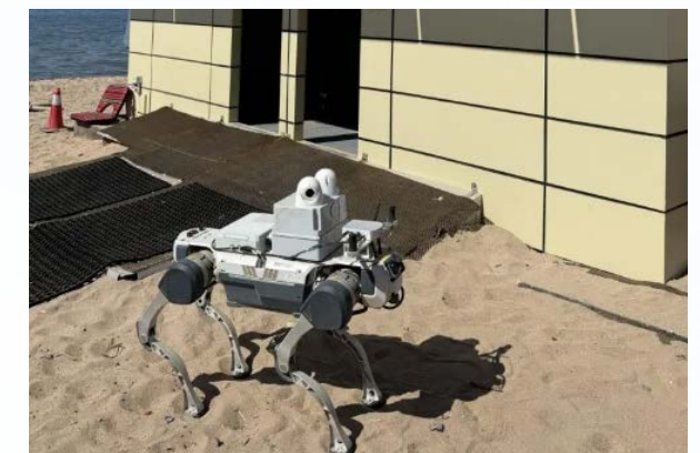
Deep Robotics' Jueying X30 robot dog for fully automatic outdoor inspection 雲深處絕影 X30 機器狗全自動戶外巡檢
