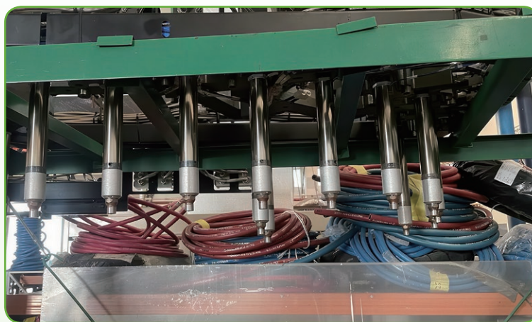
The large-scale use of hot runner systems reduces injection molding waste, improves injection molding yield, and reduces the generation of injection molding waste at the source 大規模使用熱流道系統，減少注塑流道廢料，提升注塑良率，從源頭減少注塑廢料的產生
