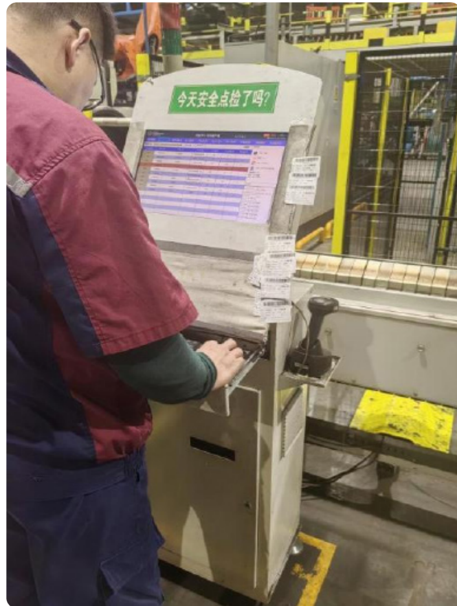
Manufacturing Execution System (MES) system integration enables electronic work instructions, reducing waste and improving efficiency
