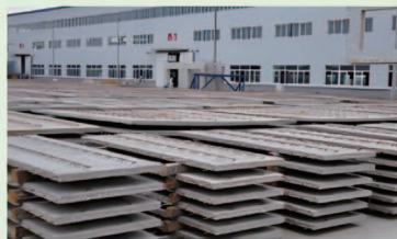
Prefabricated floor slabs
