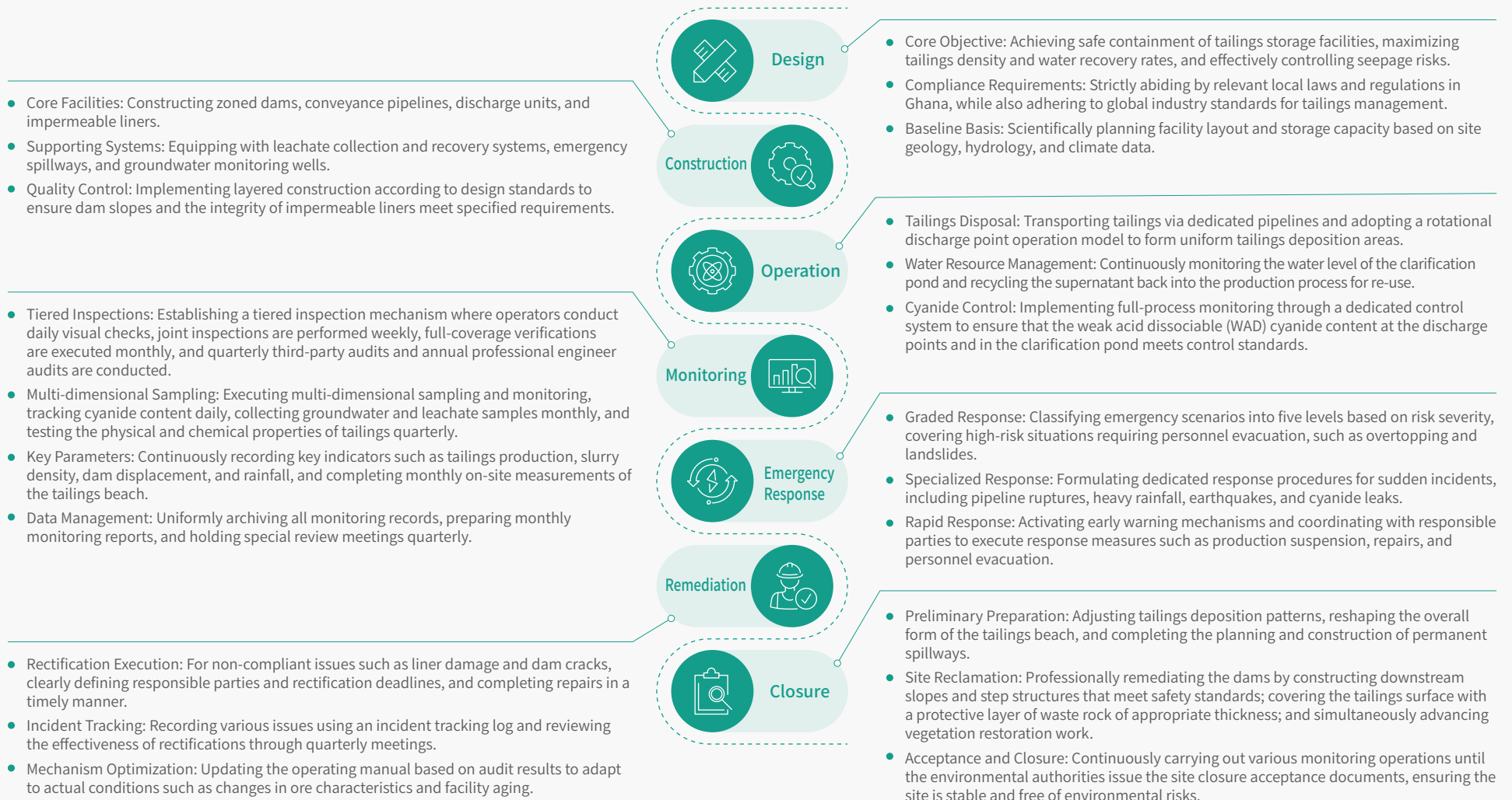
Tailings Storage Facility Management Process (Using Akyem's Relevant Regulations as an Example)
