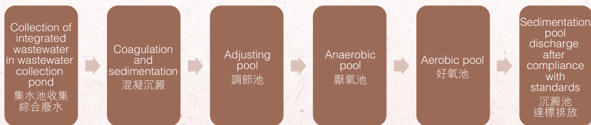
Workflow of Wastewater Treatment System of Gushengtang 固生堂污水處理系統工作流程
