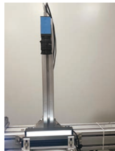
Optical fibre color ring online detection device
