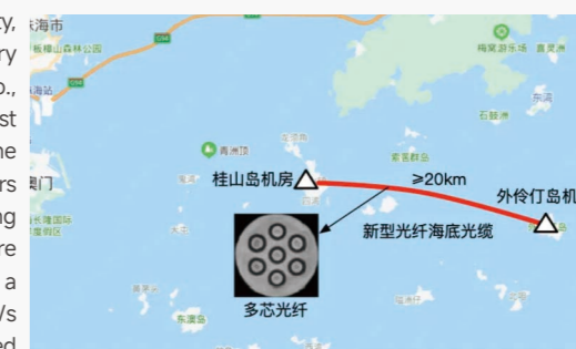
• Guishan Island - Wailingding Island space division multiplexing optical fibre submarine cable line
