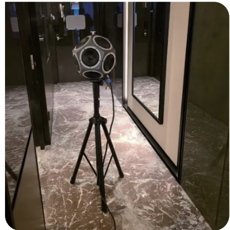
Picture: Professional acoustic measuring equipment for sound insulation testing of building components, ensuring project quality and environmental compliance
