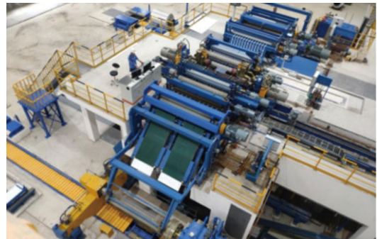
2,300mm aluminum strip high-speed trimming line
