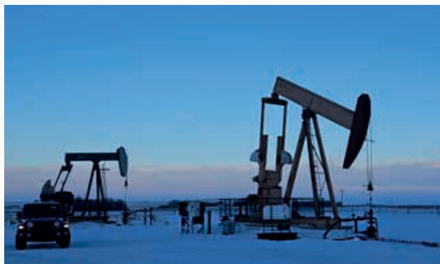
Pumping unit of well pad
